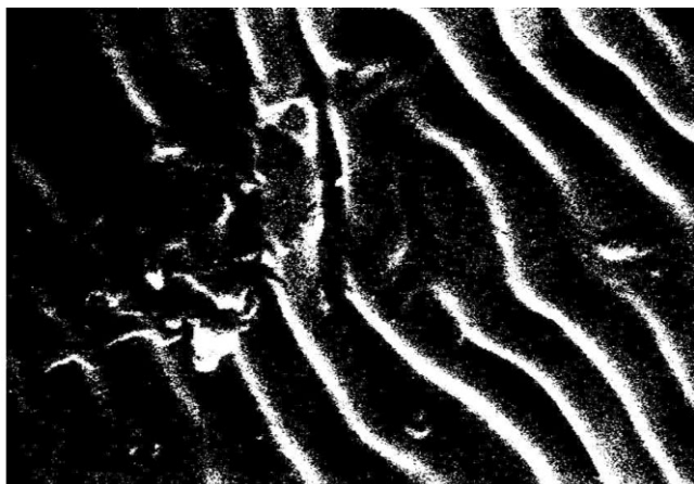
Figure 4 Electron microscopic pictures of the polyester containing 10% p -HBA.
